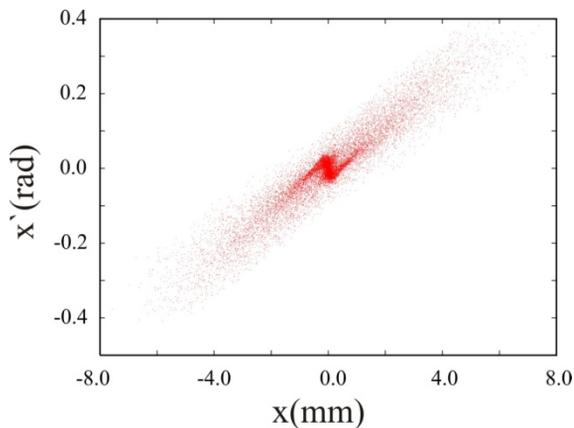
Figure 3: The x-x' phase space projection of the transported proton spectrum at 460 ps (2 cm after the target).
