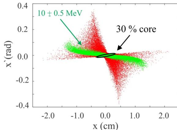
Figure 4: x-x' distribution for the proton bunch (10 ± 5 MeV) after solenoid and 6 cm drift (Red). Green marked area corresponds to the energy of interest (10 ± 0.5 MeV).
