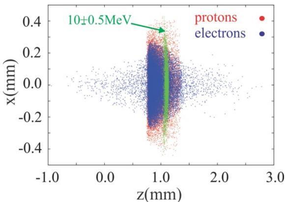
Figure 1: The proton and electron bunched in z-x plane after 25 ps after the generation in the fringing fields.
