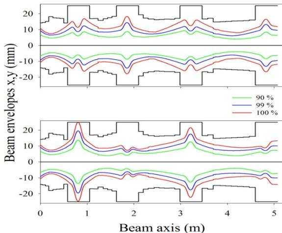
Figure 7: Transverse 90%, 99% and 100% beam envelopes starting at 6 cm from the end edge of the solenoid.
