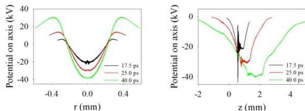
Figure 2: Potential curves in longitudinal (left) and transversal (right) directions at different positions along z.
