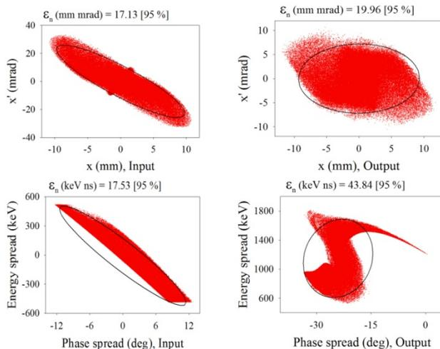
Figure 8: Transversal (up) and longitudinal (down) particle distribution at entrance (6 cm from the end of the solenoid) and exit of the CH-DTL structure.
