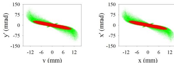
Figure 6: The cutted distributions in x-x' (left) and y-y' (right) that are fitted into the acceptance of the CH-structure. The green one shows the whole proton distribution of energy 10 MeV ± 0.5 MeV, while the red one shows the accepted distributions.
