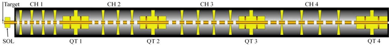
Figure 5: 3D view on the new CH- DTL consisting of four RF- cavities separated by triplet quadrupole which is suggested for the laser generated protons.
