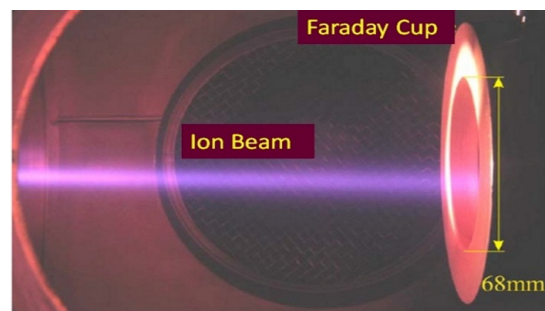
Figure 2: Photo of the 40 keV, 200 mA proton beam in front of the test stand Faraday cup (280 mm from extraction system).
