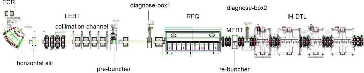
Figure 2: Layout of SSC-LINAC.
