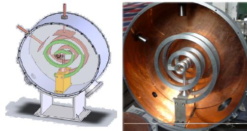
Figure 9: Structure of re-buncher.
