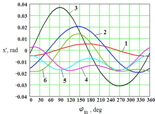
Figure 2: Effect of initial phase and lens length to the transverse motion.
