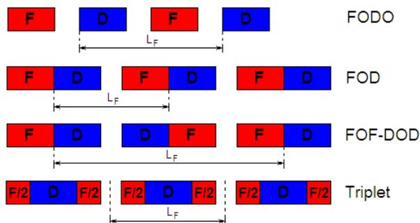
Figure 1: Some variants of static quadrupole lattices.
