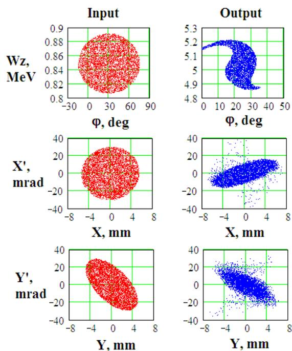
Figure 4: The longitudinal and transverse phase spaces of beam at input (red) and output (blue) of the linac.
