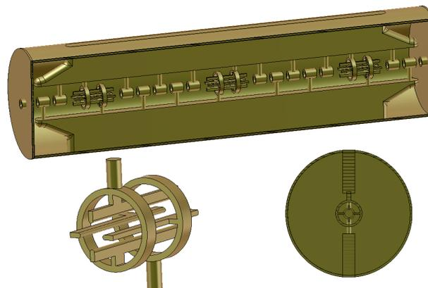
Figure 5: Schematic 3D – model of the IH – resonator with RF quadrupoles.
