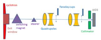
Figure 1: Elements constituting a typical basic beamline. Here an alumina foil (AlO3) is located at the end-station.
