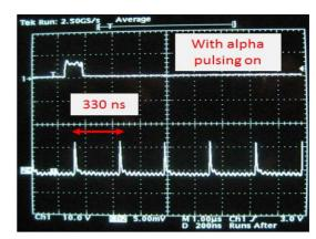
Figure 6: Bunch spacing (330 ns) with the RF deflector.
