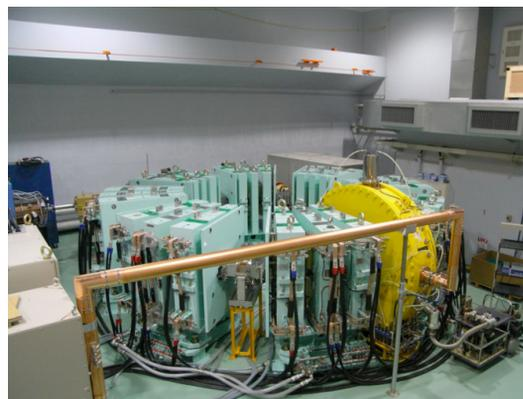
Figure 7: Photo of FFAG-ERIT compact neutron source.
