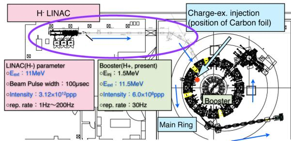
Figure 5: Schematic layout of the  $H^-$  ion injection system.
