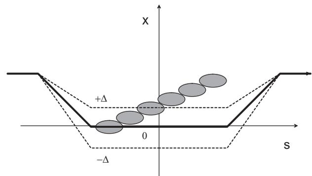
Figure 1: Trajectories at CP with positive (+ $\Delta$ ), negative (- $\Delta$ ), and zero deviation of electron energy.
