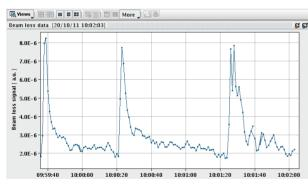
Figure 5: Closing the primary collimators to  $5\sigma$ . Loss rates recorded as a function of time for three  $10 \,\mu m$  (or  $0.036\sigma$ ) steps, in 90 m operation at the 20 October 2011 at 10:02.
