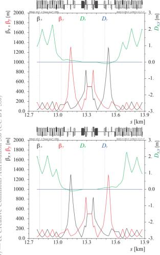
Figure 2: 500 m optics in IP5. Up for Beam 1 and down for Beam 2.
