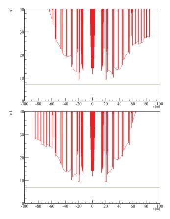
Figure 3: Aperture at 4 TeV, for the design emittance  $\epsilon_{\rm N} = 3.75 \,\mu{\rm m}$  at  $\beta^* = 500 \,{\rm m}$  around IP5 including  $\pm 2 \,{\rm mm}$  parallel separation. Top is for beam 1 and bottom for beam 2.
