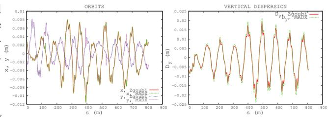
Figure 7: Left : closed orbit in AGS as stemming from alignment survey data. Right: vertical dispersion.
