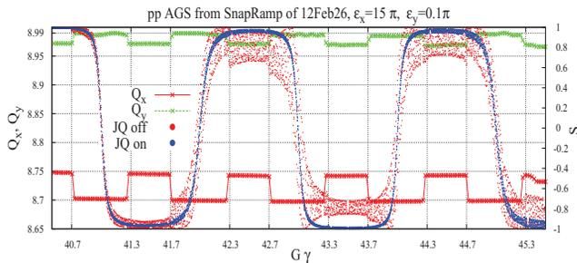
Figure 6: Spin motion with (blue) and without (red) tune jumps. Tune jumps at  $G\gamma \pm Q_x = \text{integer}$  are also shown.
