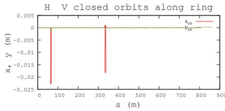
Figure 1: Zero closed orbit with local orbit bumps at snakes, injection  $G\gamma = 4.5$ . The bumps decrease to less than 2 mm at extraction  $G\gamma = 45.5$ .
