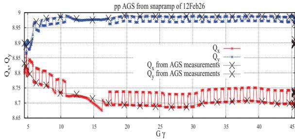
Figure 5: Simulation of tune jumps over AGS cycle (there is no tune jump in the  $\gamma_{tr}$  region).
