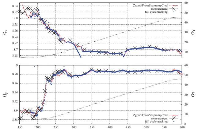
Figure 4: Tune scans over full AGS acceleration cycle, horizontal (top) and vertical (bottom).
