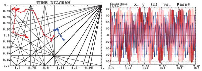
Figure 3: Left : tune diagram, including actual, measured, AGS cycle (red) and a simulation, single particle moved onto the  $Q_x - 2Q_y$  resonance line (blue). Right : in the latter case, coupled motion as the particle stands on the  $Q_x - 2Q_y$  line.
