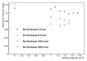
Figure 3: Number of good muons reaching the end of the muon front end cooling channel for various chicane angles and Be plug thicknesses. Note that for the 0 thickness, 0 angle case, two muon yields are listed; the '+' point is for an idealized lattice simulation, while the '\*' point and all other points are for a more realistic coil geometry.
