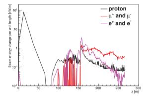
Figure 1: Total energy change of different particle species in the muon front end in the absence of a particle selection system, including gains and losses due to RF.
