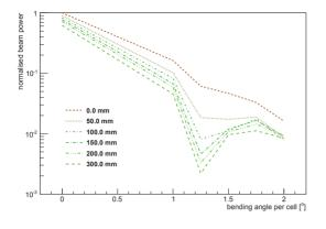
Figure 2: Total beam power of protons passing through the particle selection system, normalised to the case where particle selection system is in place.
