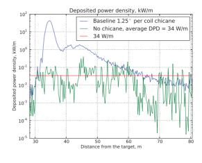
Figure 5: Deposited power density, kW/m, drift channel only, no subsequent cooling section, with and without chicane.
