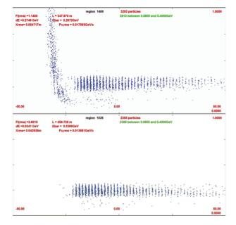
Figure 4: Phase–momenta distributions of simulated  $\mu$  beam at the end of the cooling channel. Vertical scale 0 to 1000 MeV/c; horizontal is  $c\tau$  (-50 to 50 m); (top) without chicane/absorber; (bottom) with chicane/absorber.
