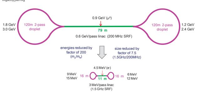
Figure 1: Schematic layout of a GeV-scale muon RLA with two-pass return arcs. A path to an 'electron model' is outlined: scaling 3.6 GeV muon RLA to 18 MeV model and replacing 200 MHz RF with a 1.5 GHz CEBAF cavity.
