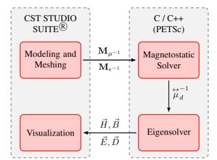
Figure 2: Strategy for the computation of eigenmodes of ferrite-loaded cavity resonators.
