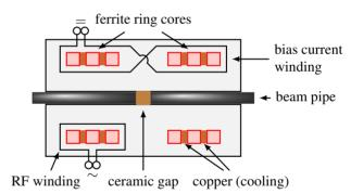
Figure 1: Simplified sketch of the main components of the SIS 18 ferrite cavity.
