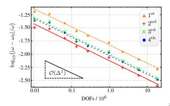
Figure 3: Relative deviation of the numerically obtained value  $\omega$  to the analytical result  $\omega_0$  as a function of the degrees of freedom (DOFs) for the four lowest eigenfrequencies for a lossless, ferrite-filled cylindrical cavity resonator.
