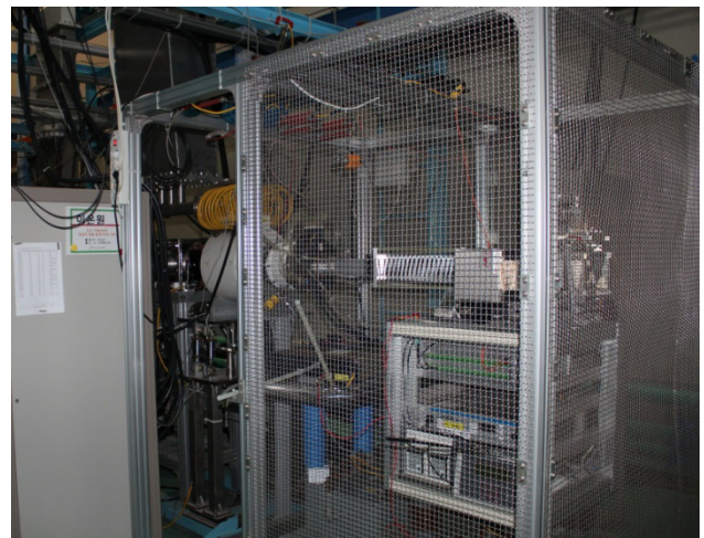
Figure 2: Installation of multi-layer DC break on the microwave ion source.
