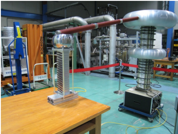
Figure 3: High voltage test of a multi-layer DC break.
