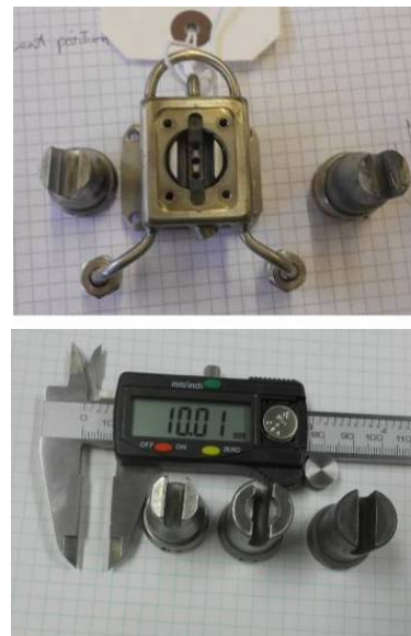
Figure 1: Modification of ISIS PD SPS: (Top) right-standard cathode with a discharge gap d=5 mm; left-modified cathode with gap d=7 mm; central-PD SPS assembling with modified cathode gap d=9 mm and the cathode modification with a drilling a cylindrical extension of the working cathode gap (bottom).
