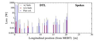
Figure 6: Beam losses for the  $90^{\circ}$  *Pair Scheme*. The collimators must absorb as mush as a few hundred Watt to reduce the losses to the level of the no halo case.
