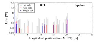
Figure 7: Beam losses for the *Single Scheme*. Each collimator only needs to absorb 10 W unlike the case of the  $90^{\circ}$  *Pair Scheme*.
