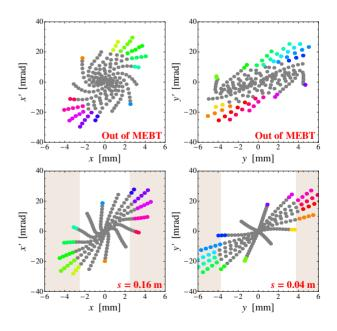
Figure 5: Sample particles ending up beyond  $5\sigma$  at the end of the MEBT (top) and their phase space positions at the proposed collimator locations for the *Single Scheme* (bottom). Brown parts represent the collimator plates.
