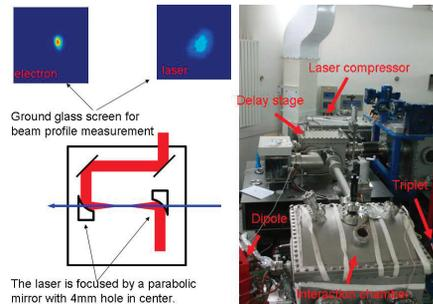
Figure 1: Layout of the interaction region of TTX.
