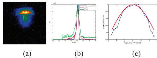
Figure 6: x-ray spectrum measurement. (a) The image from the CCD camera with 15mm thick silicon. (b) The reconstructed spectrum compared with the simulation for the centre region. (c) The measured mean energy as a function of the observation angle. The blue points were reconstructed results, the red line were the theoretical predictions.
