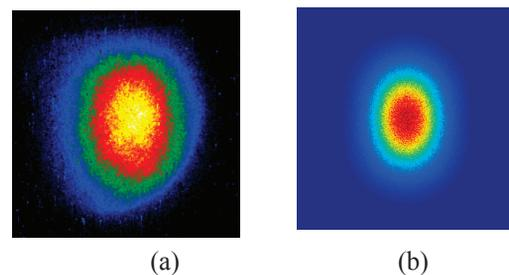
Figure 3: (a) X-ray profile measured with CCD. The left-bottom edge is cut by the Ti window; (b) X-ray profile simulated by CAIN.
