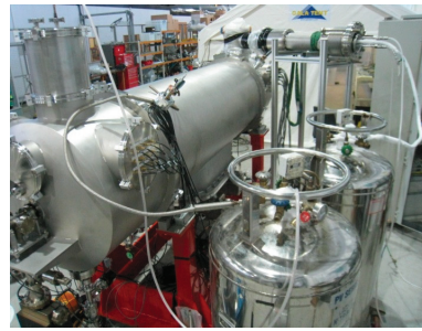
Figure 6: The Daresbury International Cryomodule undergoing final cold testing prior to installation on ALICE.
