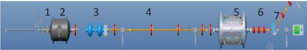
Figure 2: The layout of the CEC PoP experiment electron beam driver: 1) Cathode interchange lock-load mechanism; 2) 112 MHz SRF gun in cryomodule; 3) 500 MHz NC bunching cavities; 4) solenoids; 5) 704 MHz 5cell SRF linac in Cryomodule; 6) quadrupole magnets; 7) dipole magnet.
