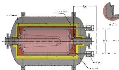
Figure 1: Cross-section of 112 MHz SRF gun with proposed modification. Two tuners will be added for precise setting of the resonant frequency.
