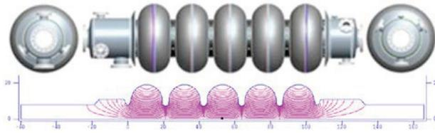
Figure 3: BNL3 20 MeV 704 MHz SRF linac and result of SUPERFISH field simulation.
