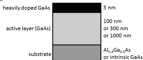
Figure 1: Crystal structure of thickness controlled photocathodes.
