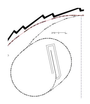
Figure 1: Layout of the injection system for SIRIUS storage ring.
