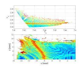
Figure 3: Frequency map of the Booster obtained from tracking of two thousand turns. Scale goes from blue, equivalent to change of  $10^{-12}$  in tune, to red,  $10^{-2}$ .
