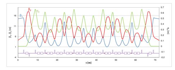
Figure 2: Optical functions of one super-period of the Booster.
