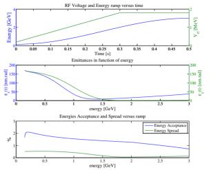
Figure 6: Evolution of emittances and energy spread in function of energy ramp of the Booster.
