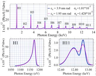
Figure 2: Flux calculation with SRW for U20 through an aperture  $0.1 \times 0.1 \ mm^2$  located at 10 m from the source.
