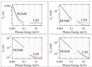
Figure 3: Beam size calculation with SRW for HU640 and U20. Red: with RW. Black: without RW
