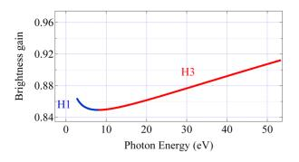
Figure 4: Calculated brightness gain using SRW versus photon energy for HU640.
