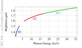
Figure 5: Calculated brightness gain using SRW versus photon energy for U20.
