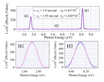
Figure 1: Flux calculation with SRW for HU640 through an aperture  $0.1 \times 0.1 \ mm^2$  located at 10 m from the source.
