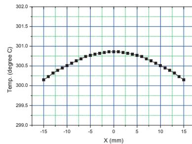
Figure 5: Temperature along magnet blocks.
