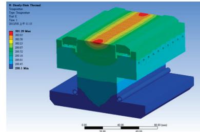
Figure 3: Temperature distribution on magnet blocks.
