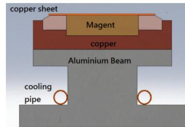
Figure 1: Magnet holder for TPS IU.
