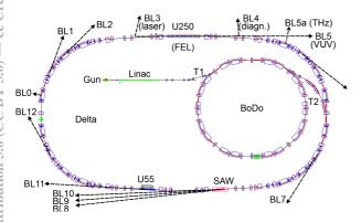
Figure 1: Sketch of the DELTA facility including the laser beamline (BL3), diagnostics beamline (BL4), VUV beamline (BL5), and THz beamline (BL5a).
