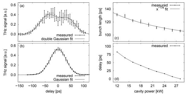
Figure 2: THz signal versus delay between the laser pulses and the electron bunch (a) with and (b) without an RF phase modulation. The square root of the THz signal is directly proportional to the longitudinal electron density. The dependence of the bunch length (c) and the synchronous phase (d), here in time units, on the RF power is studied using such profile measurements.
