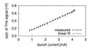
Figure 4: Square root of the THz signal versus single-bunch current.
