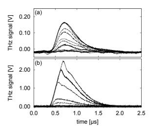
Figure 6: Oscilloscope traces of laser-induced THz signals with moderate amplitude (a). The different traces were recorded by reducing the spacial overlap between laser pulses and electron bunch. At THz signals with higher amplitude, a saturation effect in terms of a constant rising edge steepness is visible (b).
