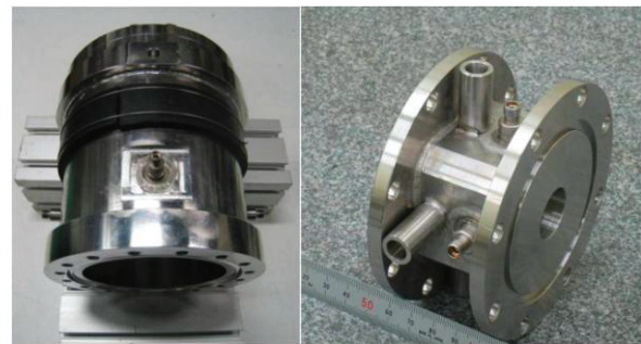
Figure 2: Photo of the beam line BPM (left) and Linac BPM (right).
