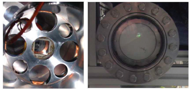
Figure 3: Left: internal view of the test stand, showing the SEM-Grid and the electron gun at the back. Right: beam spot impacting over one of the wires of the grid.
