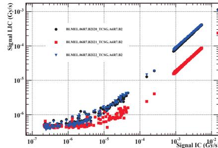
Figure 7: Signal in LIC detectors in 1.3 s vs signal observed in IC detector during the same time.
