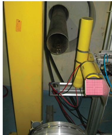
Figure 1: Detector setup in the PSB dump line. The beam direction is from bottom to top intercepting first the ceramic plate, then the LIC and finally the IC.
