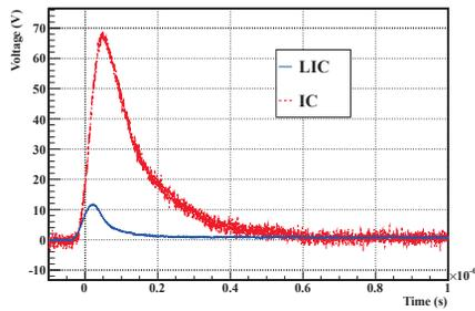
Figure 2: Electron induced signal in the ionization chambers for a beam of  $8.2 \cdot 10^9$  protons.
