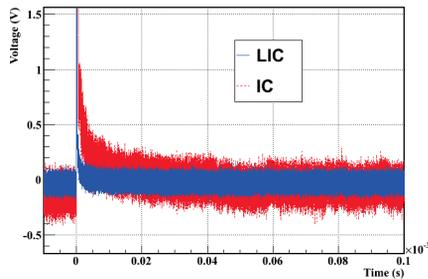
Figure 3: Ion induced tail in the ionization chambers for a beam of  $7.5 \cdot 10^9$  protons.
