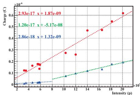
Figure 4: Charge collected in 700 ns vs intensity for IC (red circles) and LIC (blue triangles) detectors.
