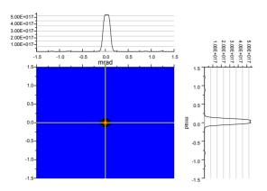
Figure 2: TPS EPU48 first harmonic photon flux contour  $K_v = 4$ ,  $K_x = 2.64$ .
