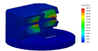
Figure 5: TPS EPU48 XBPM temperature contour when  $K_x = 1.6$ ,  $K_y = 0.8$ .
