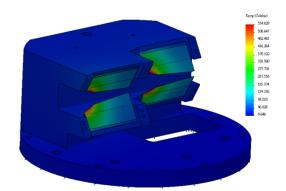
Figure 4: TPS EPU48 XBPM temperature contour when  $K_v = 4$ ,  $K_x = 2.64$ .
