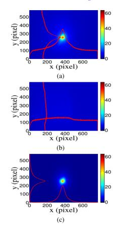
Figure 3: Background subtracted to minimize impact of dark current; (a) a beam with the dark current and background noise, (b) a background image, (c) a beam image when dark background was subtracted.
