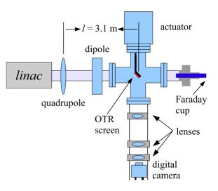
Figure 1: Apparatus used to measure the beam emittance.
