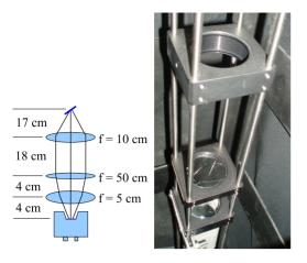
Figure 2: The OTR Imaging system.
