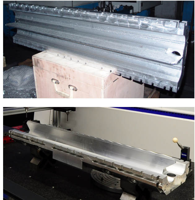
Figure 2: a: Major vane during machining phase, after first rough machining at Mecanizados Mandrinados Mancisidor . b: Same vane at the Zeiss metrology lab.
