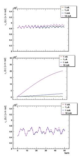
Figure 4: Evolution of (normalised) RMS emittance over 50 turns starting with a  $10 \pi$  mm mrad (unnormalized) parabolic distribution for varying beam currents, where x is horizontal (top), y is longitudinal (middle) and z is vertical (lower).
