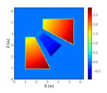
Figure 1: Magnetic mid-plane field of one cell of the FFAG design.
