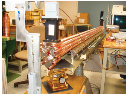
Figure 2: ALBA accelerating structure after brazing.
