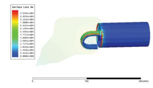
(b) RF loss density profile on the loop length of 45mm
