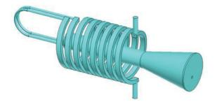
Figure 5: Schematic drawing of cooling channel at the RF input coupler tip.
