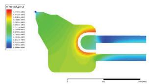
(a) Magnetic field profile around the loop length of  $L=45\,\mathrm{mm}$
