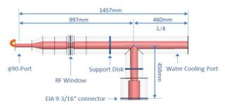
Figure 1: Schematic drawing of an RF input coupler with water-cooling port of  $\lambda/4$ .
