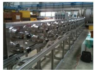
Figure 2: Photograph of real size Aluminum RFQ module; the axial length of 9.78m-long.
