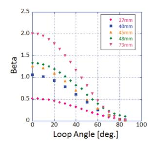
Figure 3: Evaluation of beta (RF coupling) on beam loading in IFMIF/EVEDA prototype RFQ; beta vs. Loop angle for the inserted depth of 27, 40, 45, 48 and 73mm.
