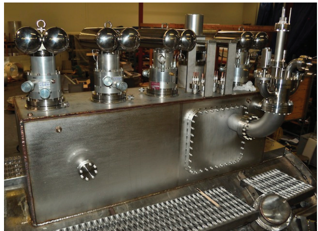
Figure 5: Completed main cryocooler tower.
