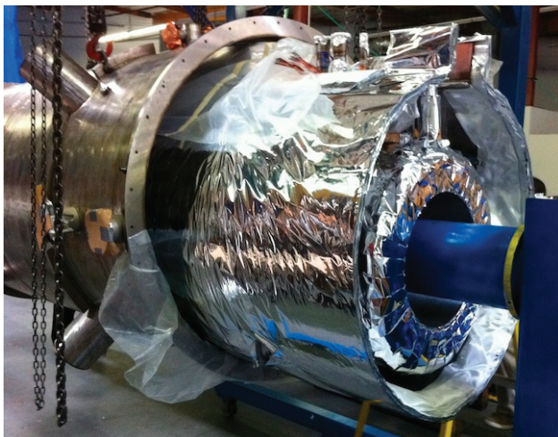
Figure 3: Assembly of shield/cold mass into cryostat.
