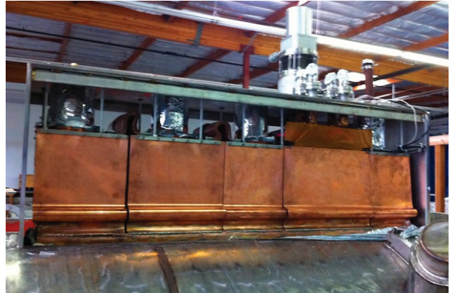
Figure 4: Improved shield connection to cryocoolers.
