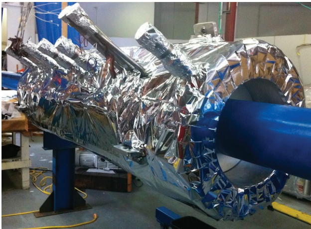
Figure 2: Cold mass after MLI wrapping.
