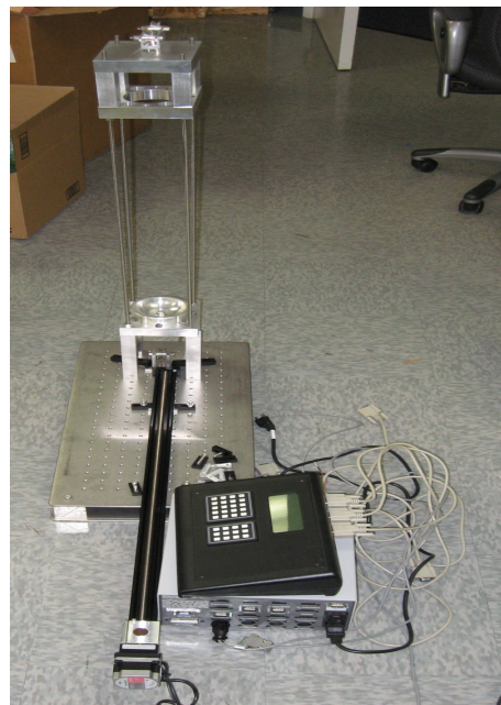
Figure 5: The bead pull fixture and motion control system.
