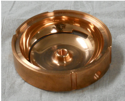
Figure 3: A finished half-cavity copper part.
