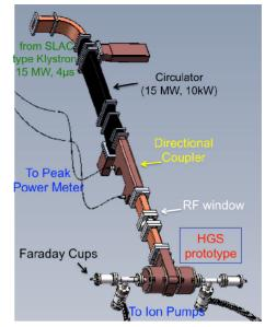
Figure 8: CAD model of the high-power RF setup.
