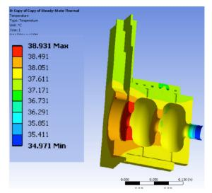
Figure 4: Temperature distribution inside the HGS.
