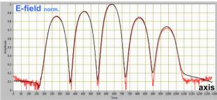
Figure 7: Axial electric field profile (bead-pull).
