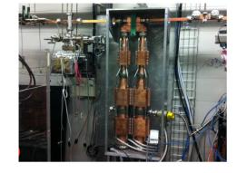
Figure 3: Pulse compressor with temperature stabilization system installed in the test stand.
