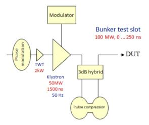
Figure 1: Lavout of the CERN X-band power source.
