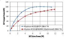
Figure 5: The comparison of drive/output power curves of klystron SN102 between NSRRC and CPI.
