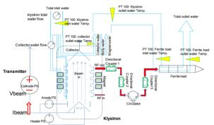
Figure 2: RF test stand for CPI 100kw klystrons with improved VSWR.
