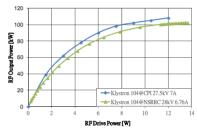
Figure 7: The comparison of drive/output power curves of klystron SN104 between NSRRC and CPI.
