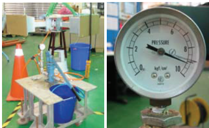
Figure 6: The water pressure persistent test stand for the repaired water leak 350kW circulators.
