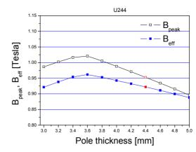
Figure 3: The dependence of the peak field and effective field on the pole thickness.
