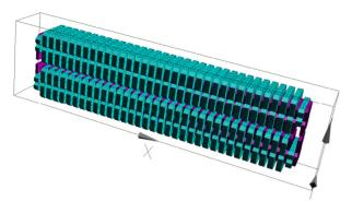
Figure 6: Shortened RADIA model of the undulator. Movable tuning magnets at the end regions are shown.
