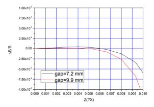
Figure 4: Transverse roll-off at minimum working gap and at maximum working gap.
