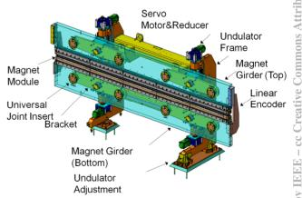
Figure 2: Schematic structure of PAL-XFEL undulator system.
