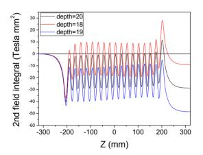
Figure 7: The calculated orbit for 3 different tuning block depth.
