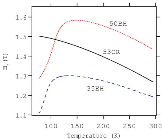
Figure 3: Temperature dependence of the remanent fields ( $B_r$ ) of sintered NdFeB magnets (35EH and 50BH) and of a PrFeB magnet (53CR), from Ref. [8].
