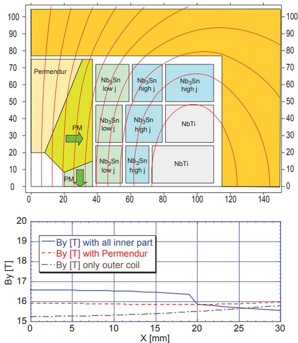
Figure 5: Block layout of an alternative higher-field Nb-Ti/Nb<sub>3</sub>Sn/PM HE-LHC dipole-magnet coil modeled with PANDIRA. The magnet is surrounded by an iron return yoke. Three calculations were carried out: (1) with outer coils only; (2) with permendur added, and (3) with all inner parts. Only one quarter of one aperture is shown. The easy axes of the permanent magnets are indicated by the green arrows.
