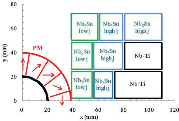
Figure 2: Block layout of a newly proposed hybrid Nb-Ti/Nb<sub>3</sub>Sn/PM HE-LHC dipole-magnet coil (modified Fig. 1). Only one quarter of one aperture is shown. The easy axes of the permanent magnets are indicated by the red arrows.
