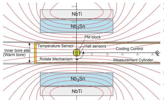
Figure 4: Setup for field-enhancement measurement.
