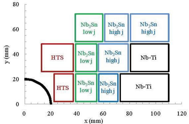
Figure 1: Block layout of the hybrid Nb-Ti/Nb<sub>3</sub>Sn/HTS dipole-magnet coil design for the HE-LHC [3]. Only one quarter of one aperture is shown.
