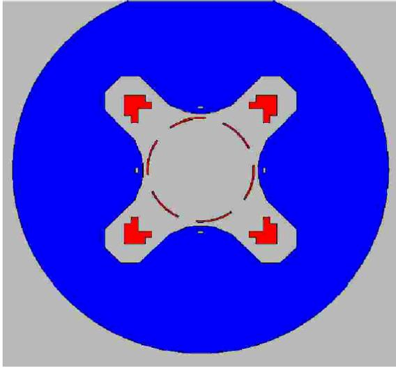
Figure 4: Sketch of the sextupole coils inserted into the BNL R&D quadrupole magnet.
