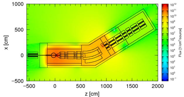
Figure 1: Radiation fluence seen in the fragment pre-selector at FRIB. The figure is from [1].
