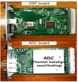
Figure 5: DSP and ADC board of controller.
