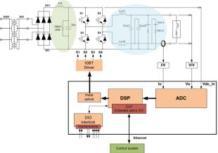
Figure 3: Circuit diagram of bipolar MPS.
