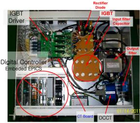
Figure 4: Fabricated bipolar MPS.
