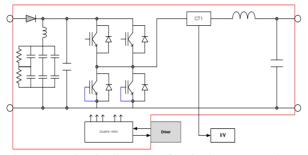
Figure 2: Circuit diagram of unipolar MPS unit stack power supply.
