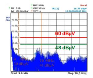
Figure 7: Reduction of conducted EMI intensity after offline UPS installation.
