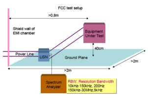
Figure 2. Experimental apparatus.
