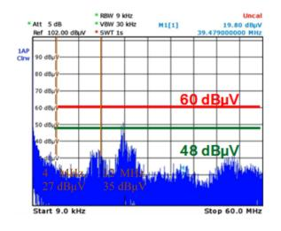
Figure 6: Reduction of EMI intensity after filter added.
