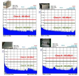
Figure 3. Conducted EMI spectrum of some qualified power supplies.
