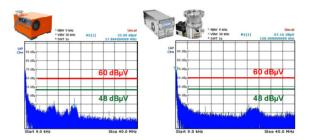
Figure 4: Conducted EMI spectrum of different kinds of vacuum pumps which conform to class B.
