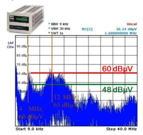
Figure 5: Dual controller of ionization pumps emits obvious noise.
