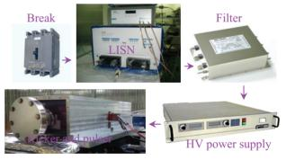
Figure 6: Experimental setup with EMI filter.
