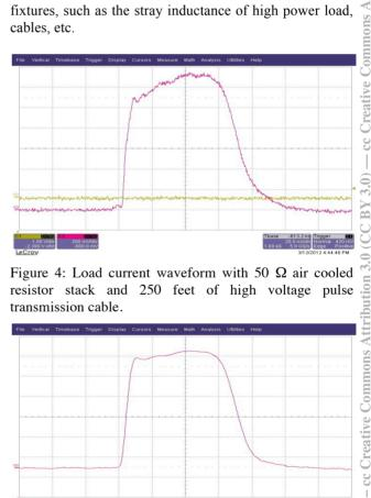
Figure 4: Load current waveform with 50  $\Omega$  air cooled resistor stack and 250 feet of high voltage pulse transmission cable.
