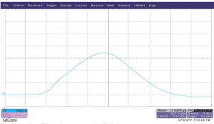
Figure 9: The integrated field measurement of kicker magnet with 25 ohm load at 40kV.
