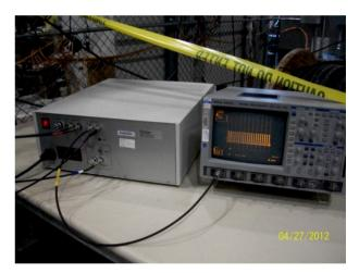
Figure 2: FID pulse generator under 50 kV, 1 kA, and 100 Hz test.
