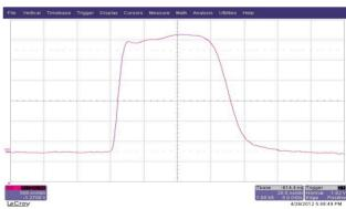
Figure 5: Load current waveform with 50  $\Omega$  oil cooled resistor stack and 250 feet of high voltage pulse transmission cable.
