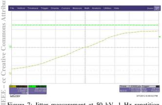
Figure 7: Jitter measurement at 50 kV, 1 Hz repetition rate.
