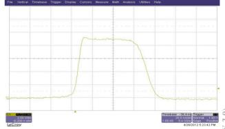
Figure 3: FID voltage monitoring output waveform at 50 kV.
