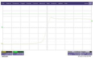
Figure 8: Jitter measurement at 50 kV, 100 Hz repetition rate.
