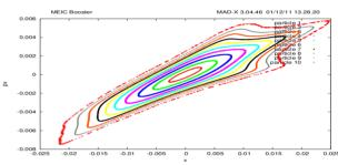
Figure 7: Ten orbits started at 1 through 10 standard deviations radially in horizontal phase space. They are advanced through 1000 turns to examine orbit stability.
