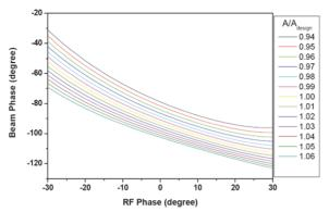
Figure 5: Beam phase as a function of RF phase for DTL103.
