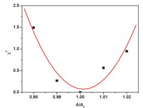
Figure 4: Amplitude determination by comparing the simulation results with the artificial experimental result for the relative amplitude of 1.0.
