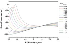
Figure 3: Beam phase as a function of RF phase for DTL101.
