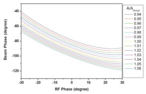
Figure 7: Beam phase as a function of RF phase for DTL104.
