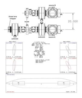
Figure 4: The LEBT has 2 H- sources but only one is used at any given time. The two sources are mounted on a slide so that either source can be slid into operation. The length of the LEBT from the end of the source to the start of the RFQ is about 1.2 m.
