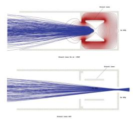
Figure 6: The magnetic field from the solenoid focuses the beam into the entrance of the RFQ when the Einzel lens is off. When the Einzel lens is on, it acts like a mirror on the
