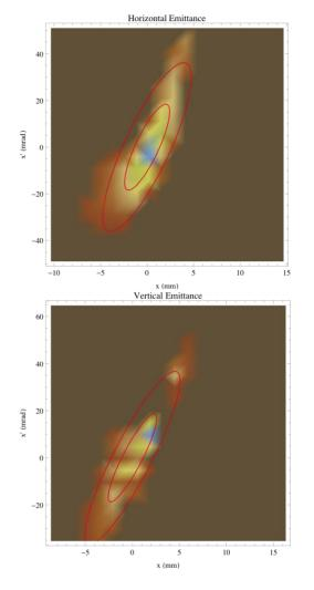
Figure 5: The horizontal and vertical emittance at the end of the LEBT.
