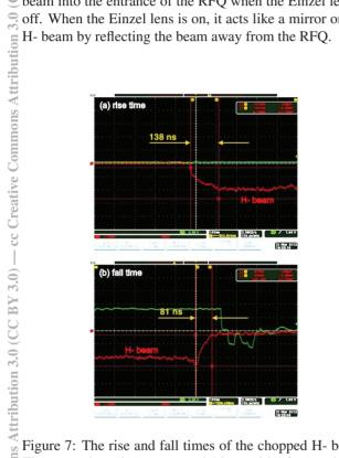
Figure 7: The rise and fall times of the chopped H- beam. The traces have been averaged  $16 \times$  and background subtracted.
