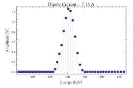
Figure 8: The energy spectrum clearly shows the mean beam energy is 700 keV for 168 kW of RFQ forward and 12 kW reflected power.
