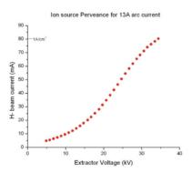
Figure 3: The perveance curve of the source shows that there is a roll off in beam current above 35 kV.
