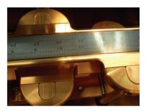
Figure 9: A rod when compared to the straight edge of a ruler clearly shows that there is a gap between the rod and the ruler.
